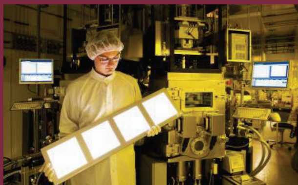
Pictures: Large Area OLED Lighting modules (left: 20x20 cm 2 , right: 80 x 20 cm 2 ) fabricated at the Fraunhofer IPMS. Copyrights: Fraunhofer IPMS
