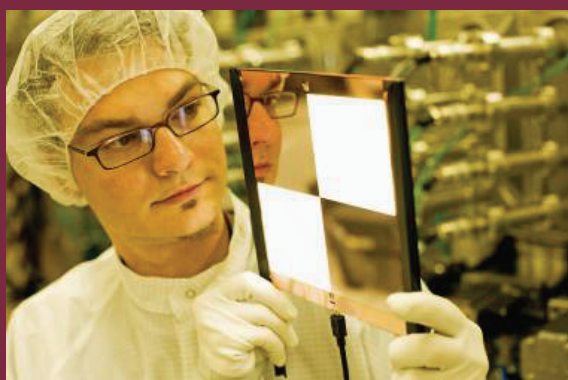
Pictures: Large Area OLED Lighting modules (left: 20x20 cm 2 , right: 80 x 20 cm 2 ) fabricated at the Fraunhofer IPMS. Copyrights: Fraunhofer IPMS
